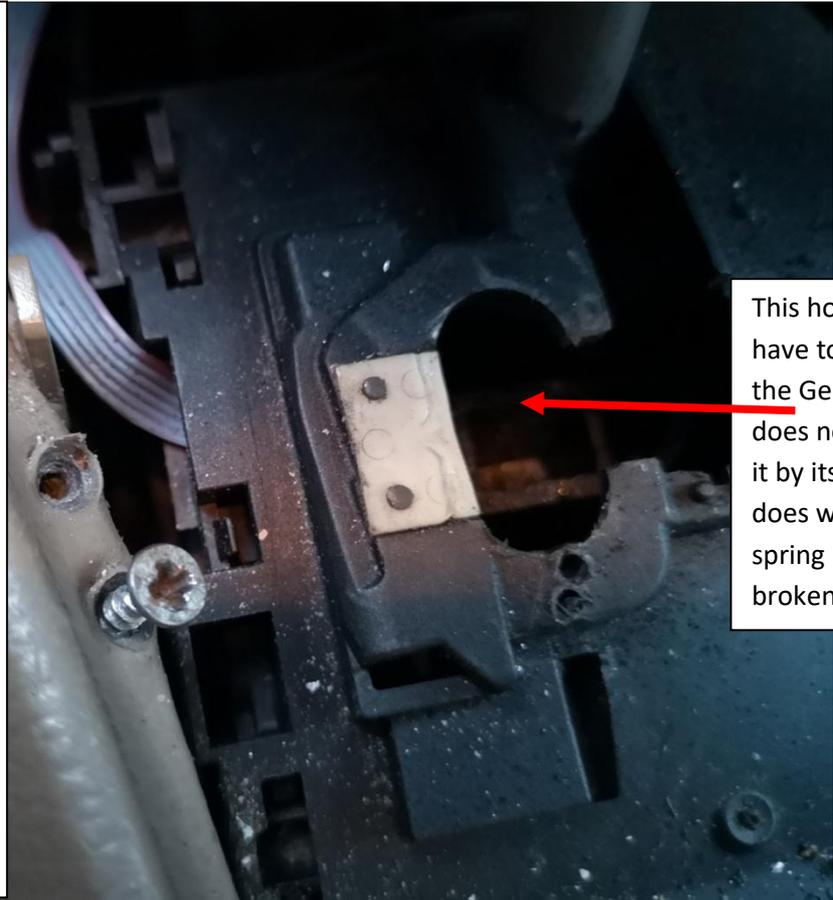
This hole you have to block so the Gear Lever does not go into it by itself as it does when the spring is broken.
