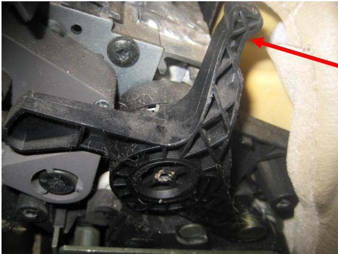
Push the screw driver in the same angel as the arrow shows and at the same time use the original push switch.
